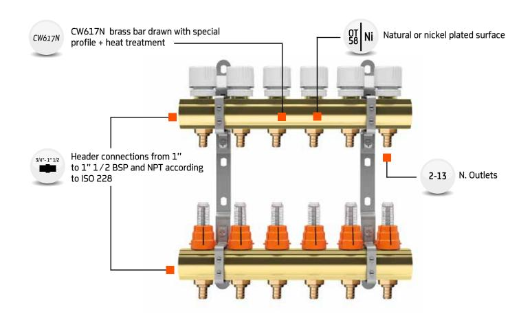
Supplied as standalone components or in flow (F) / return (R) kits; preassembled on standard or low thickness (3 5/32") brackets. Available with outlet fittings, lockshield-type (F), FLUXER (F) or thermostatic control (R) inserts.
